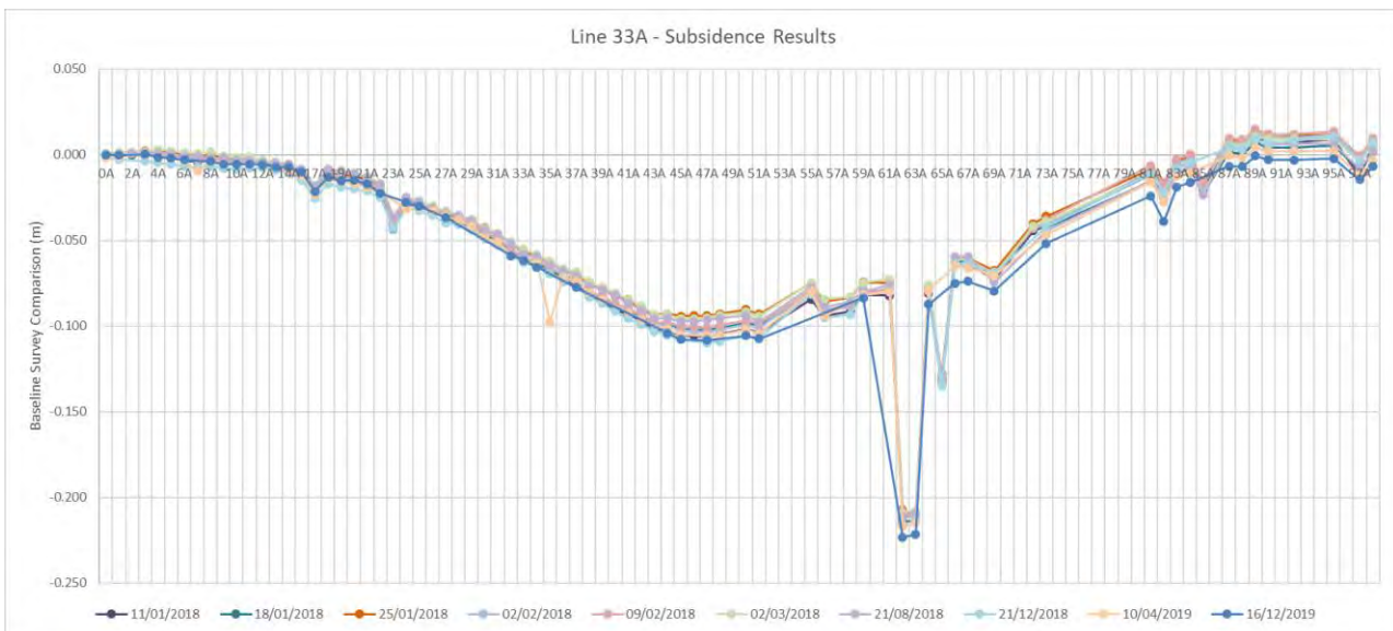
Figure 10 - Line 33A Subsidence Results
