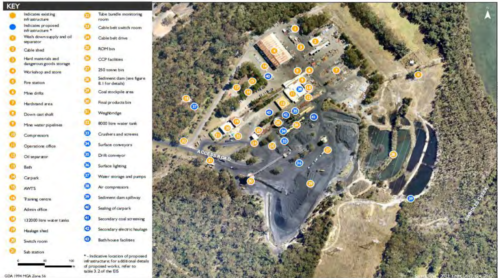
Mine pit top infrastructure elements Chain Valley Colliery Mining Extension | Project - Environmental Impact Statement Figure 2.4
